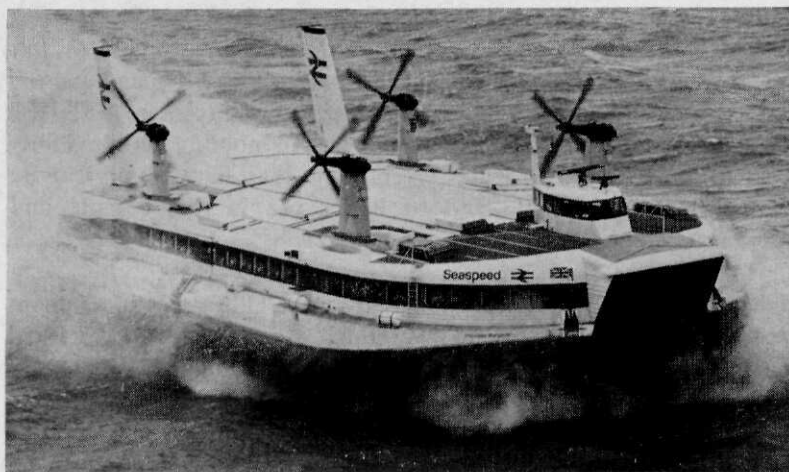
One of the SRN4s operated by Seaspeed on the Dover Boulogne route in the Channel. With a top speed of 78 knots (148 km/h) these craft would have a high reinforcement capability in time of crisis; they can carry 254 passengers and 30 vehicles
