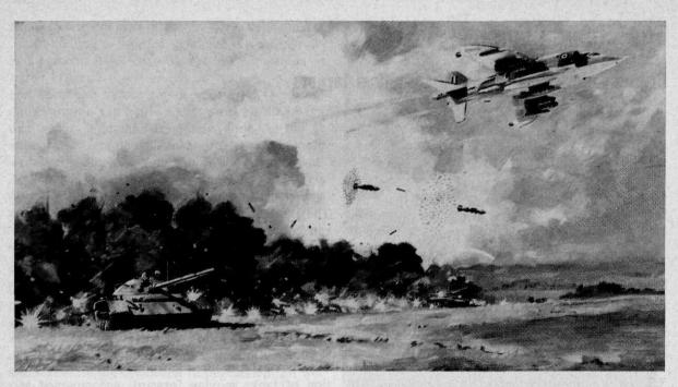
a safe separation distance between aircraft and weapon before bomblet ejection. Following release and after the set delay, skin-lifting jacks force the leading edge of the centre section into the air-stream, so that aerodynamic forces can lift the covers clear of the weapon and allow the bomblets to be ejected in a sequence.
